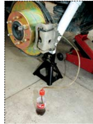
A nut is used under the wheel nut to ensure the rotor doesn't float around during bleeding operations. The correct procedure for bleeding starts with the left-hand rear, then the right-hand rear, the left-hand front and finally the right-hand front
