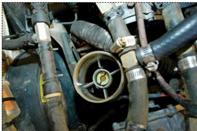
The brake fluid reservoir must be drained of old fluid and cleaned before the new fluid is used to flush the whole system
