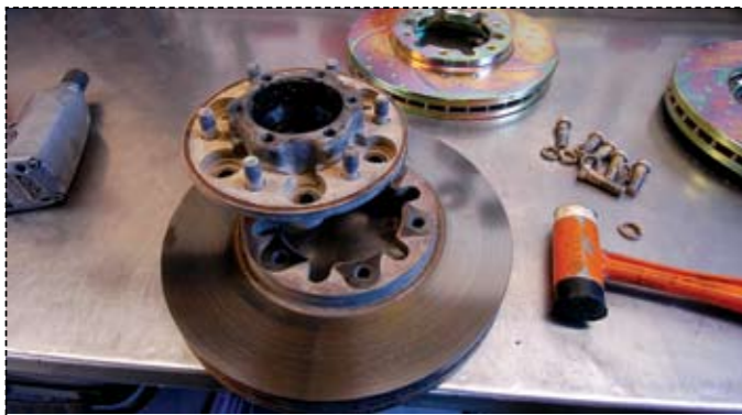
With the bolts removed, a gentle tap with a soft hammer might be required to separate the hub and disc rotor
