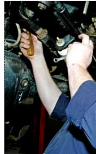
Greg Smith unclips the top, central, flexible brake line after cracking the fixed-line connection
