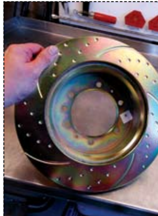
The slotted rotors from RDA come marked left or right to avoid confusion
