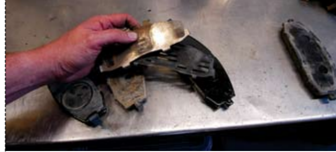
The extra plates on the old pads should be cleaned and fitted to the new pads before they are placed back in the callipers
