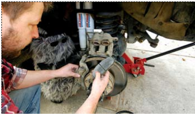
Once the centre section of the calliper is unbolted, you can get to the pads. When you remove them, make sure you don't lose the backing plates on the pads themselves. These plates prevent brake squeal and act as a buffer between the piston assembly and the pads
