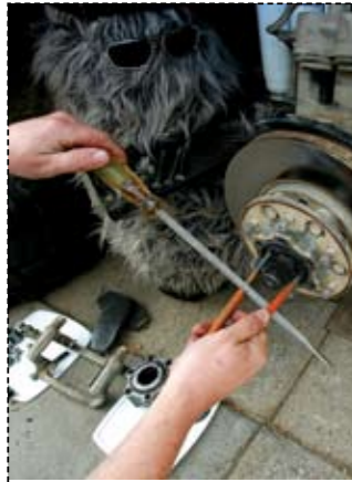
If you don't have the right tool to remove the bearings, two punches and a screwdriver will enable you to remove the bearings easily
