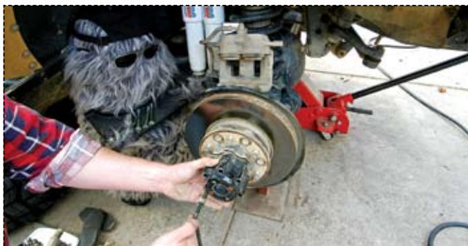
Remove the bolts that hold the hub in place
