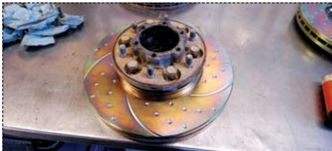
Tighten all the bolts evenly to the genuine factory specifications. Every fourby will be different here, so it will pay to check before you bolt things together
